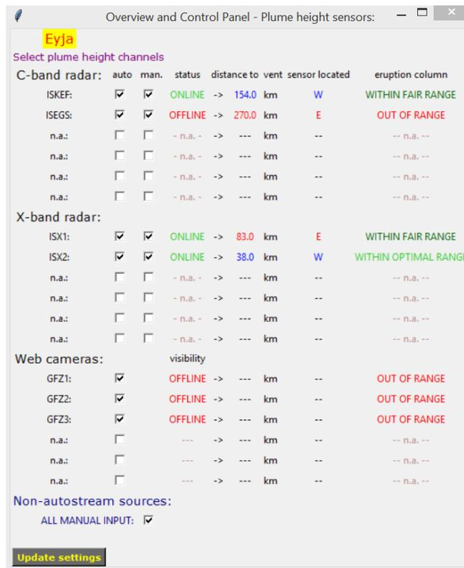
Figure 18: Plume height sensor control panel
