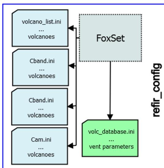
Figure 4: Content of the folder refir\_config: This folder needs to include all five mandatory “.ini” files. In addition it can contain the “.ini” file generator FoxSet.
